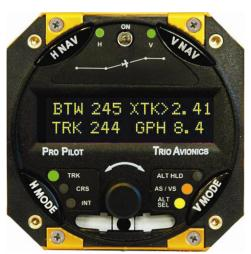
The fuel flow in **GPH** (gallons per hour) or **LPH** (liters per hour) is always available in the variable data on the bottom right quadrant of the display. Rotating the encoder knob will cycle through the GPS data screens to bring this data into view. A small momentary pushbutton, mounted to the instrument panel or control stick allows the pilot to view additional fuel parameters.
